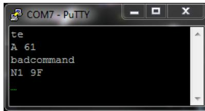
Figure 19: A command line terminal of a Servo Cylinder in Machine Mode 1 displaying a valid command followed by an ACK, and an invalid command followed by a NACK. Both acknowledgements are followed by a two-character checksum.
